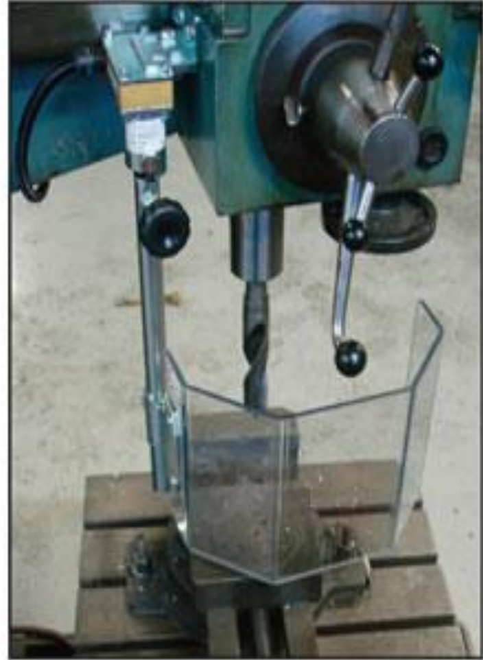
Electrically Interlocked Shield for Larger Drill Presses and Radial Drill Presses
