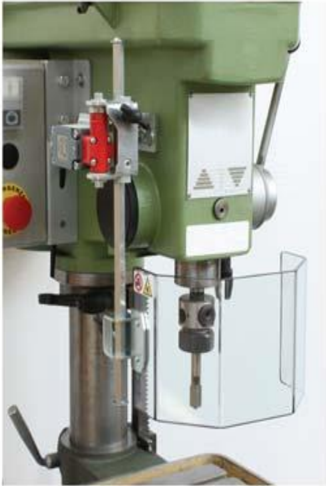
Electrically Interlocked Shield for Small to Medium Size Drill Presses
